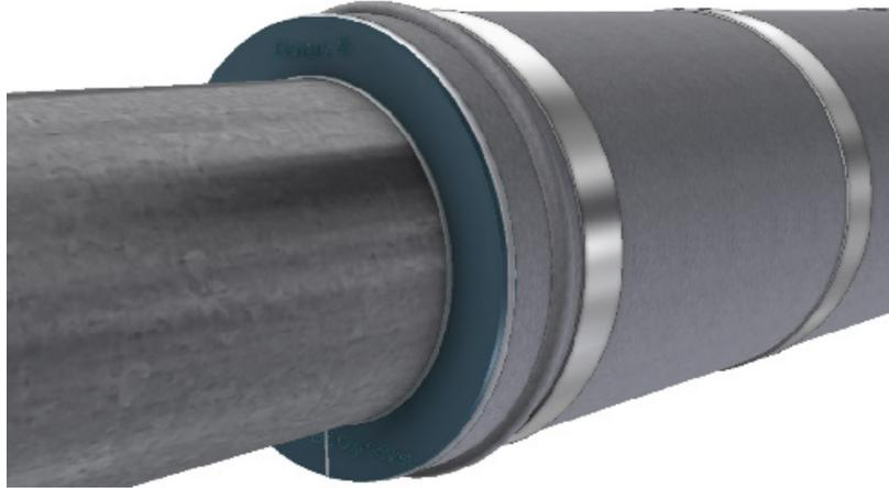
**End termination of pipe insulation is a critical point of water proofing the pipe insulation material. Preparing end termination of traditional metal insulation cladding may be challenging to achieve with water ingress as a result. Water under the insulation and potential damages to pipe coating due to sharp metal edges is major risk factor resulting in development of CUI.**
